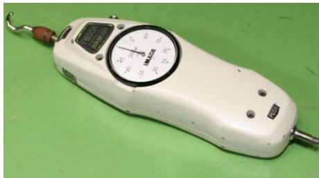
Fig. 3 Mechanical force gauge (dynamometer) Max: 500kg
